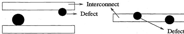
Figure 1. Not all defects cause a failure to occur.
