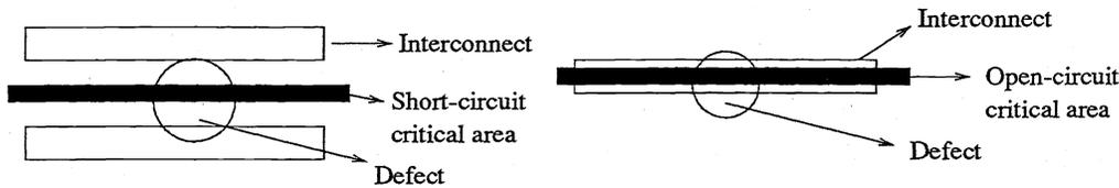
Figure 2. Defects falling on the "critical area" leading to failures.
