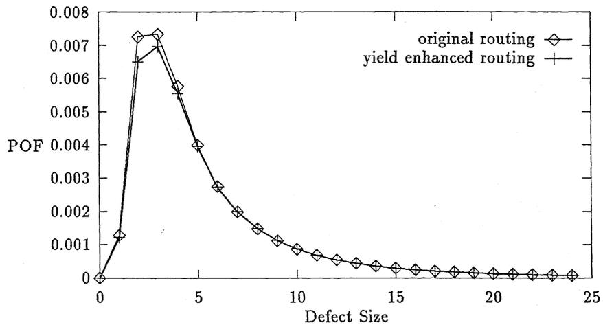
Figure 8. ex3b - Probability of Fails versus Defect-size
