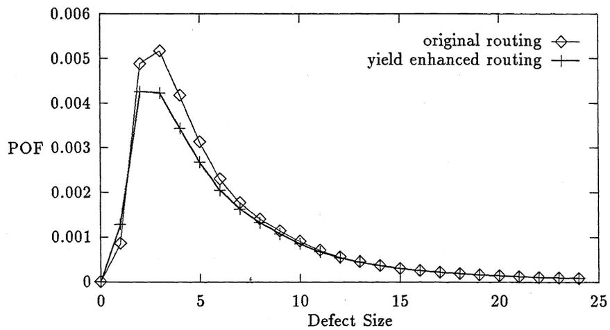
Figure 5. Example1 - Probability of Fails versus Defect-size
