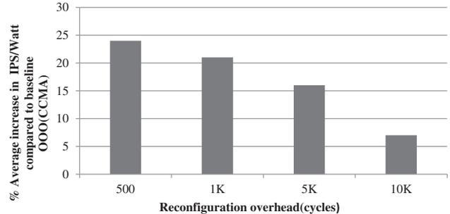
Fig. 12. Reconfiguration overhead and its impact on throughput/Watt gains.
