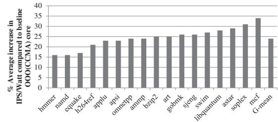
Fig. 6. % Average increase in IPS/Watt compared to the baseline OOO(CCMA) using PMC\_RPE scheme
