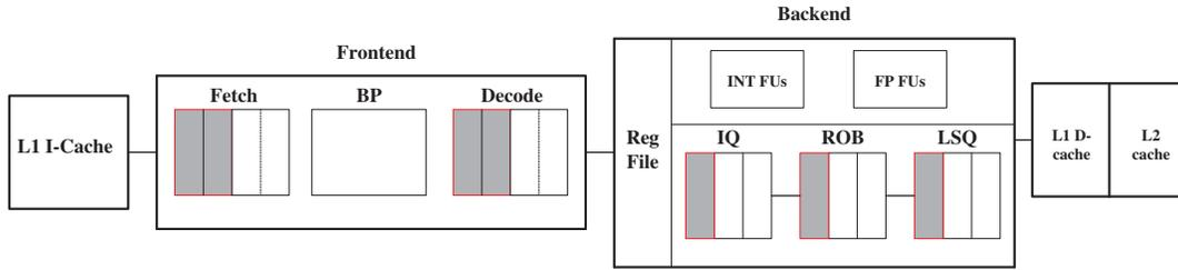
Fig. 1. High-level view of the reconfigurable architecture. The shaded units are reconfigured during run time.
