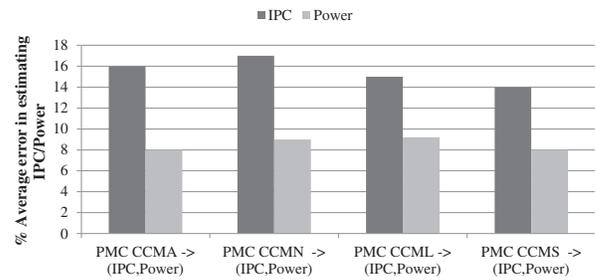
Fig. 2. Average error in estimating power/IPC across all CCMs using the PMCs of the host CCM. For example, PMC CCMA  $\Rightarrow$  (IPC,Power) denotes the average error in estimating power and IPC on all other CCMs using the PMCs of CCMA.
