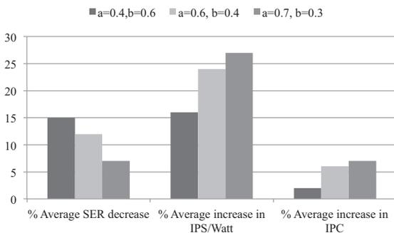
Fig. 10. Variation in Throughput/Watt, performance and Effective\_SER while switching based on PMC\_RPE scheme.
