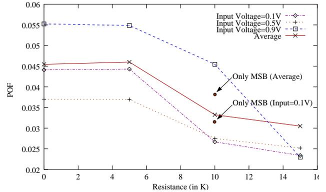
Figure 7: **Variation in sensitivity with increasing resistance (R),  $p=3, q=8, r=32$**
