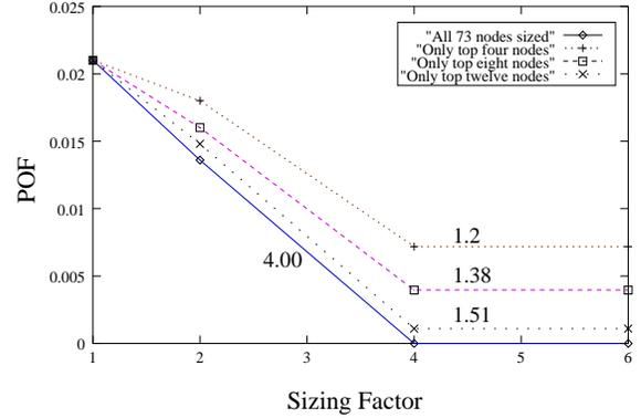
Figure 9: Sensitivity variation with selective node resizing with injection level bounded by 1pC (the number on the curves indicate the corresponding fault-sensitive area increase factor)
