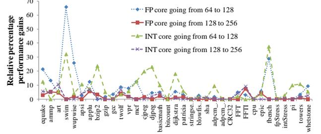
Figure 4. Ratio of the IPC for the core configurations when going from lower to higher sizes of ROB.
