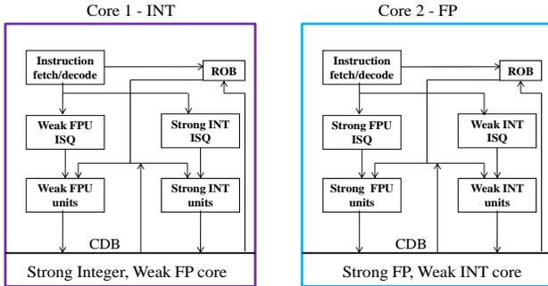
Figure 1. Baseline configuration for two heterogeneous cores.
