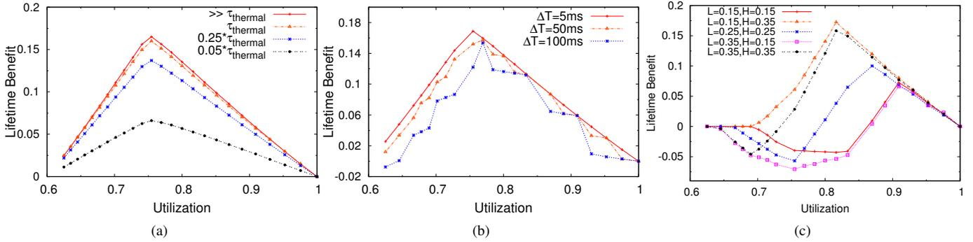
Fig. 7. (a)Benefit of WA-DVFS over P-DVFS for different phase lengths (b) Benefit of WA-DVFS over P-DVFS for different time steps (c) Benefit of WA-DVFS over P-DVFS for an inaccurate execution time estimation
