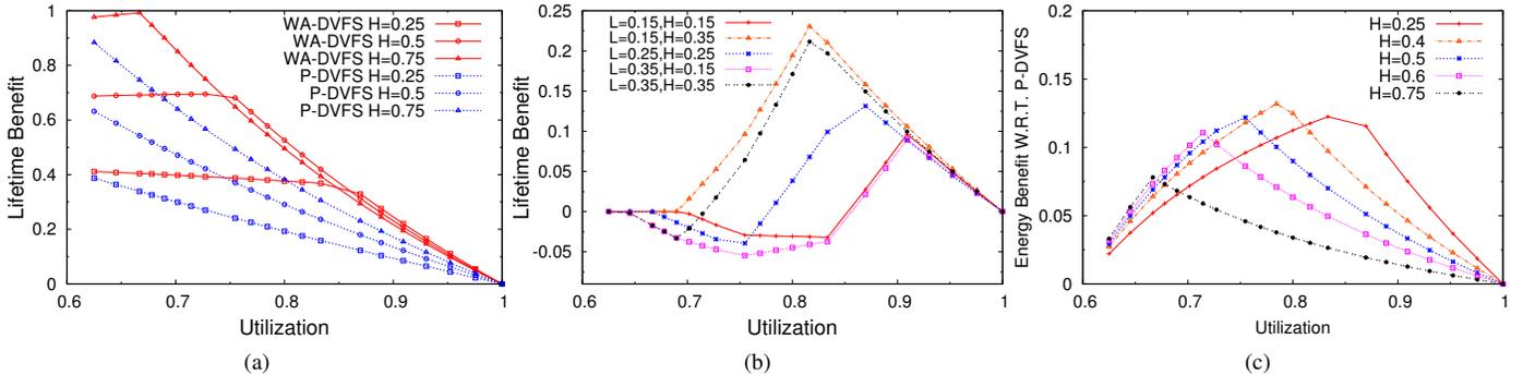
Fig. 8. (a) Benefit of WA-DVFS and P-DVFS over no DVFS using an actual benchmark workload assuming an accurate execution time estimation (b) Benefit of WA-DVFS over P-DVFS using an actual benchmark workload assuming an inaccurate execution time estimation (c) Energy saving of WA-DVFS over P-DVFS using an actual benchmark workload and assuming an accurate execution time estimation
