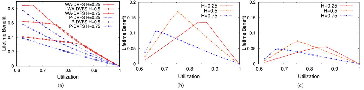
Fig. 6. Lifetime benefit of WA-DVFS over P-DVFS assuming an accurate execution time estimation: (a)Benefit of WA-DVFS and P-DVFS over no DVFS assuming an accurate execution time estimation (b) Large IPC difference (0.2 vs 2.2), (c) Small IPC difference (1.2 vs 2.2)
